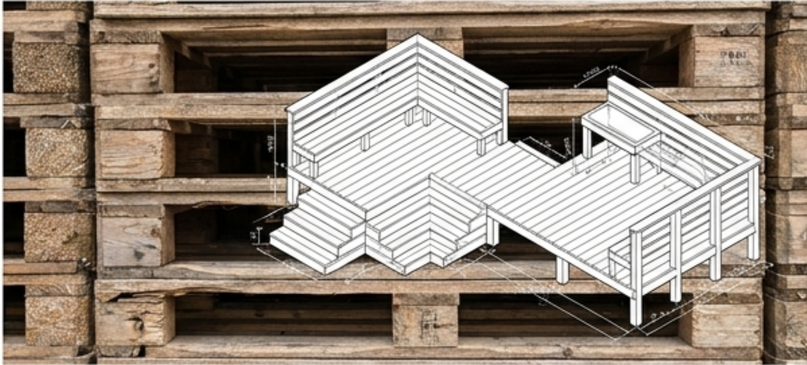
Quadrant 1 (The Europallet Economy): 100+ free pallets sourced from local logistics. Transformed into horizontal decking, outdoor kitchen worktops, and vertical privacy screens.
